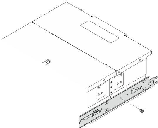
Step 5. Remove the inner rail from the server.
