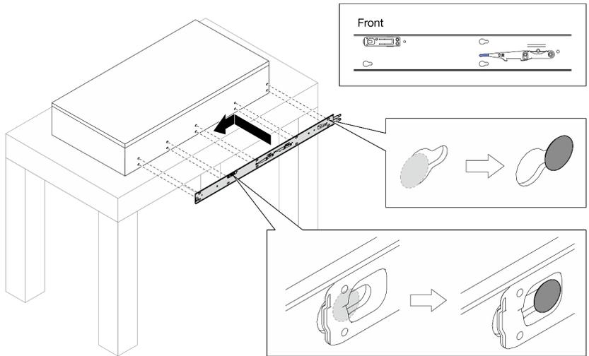
Step 4. Insert and tighten an M4 screw to secure the inner rail as shown.
