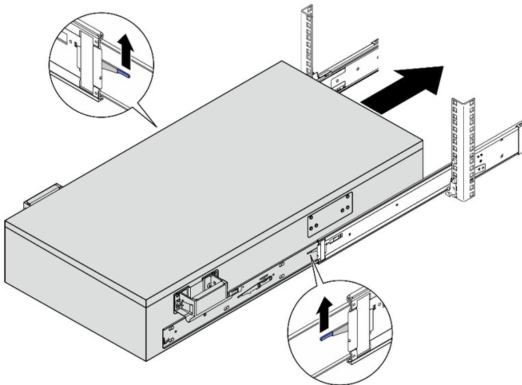
d. Remove the front lift handles.
