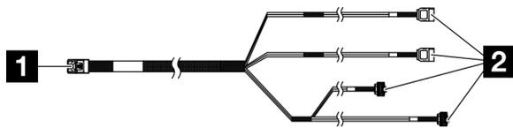
図 111. Mini SAS HD X4 Vertical to VT SATA 7P x2 + RA SATA 7P x2 cable
