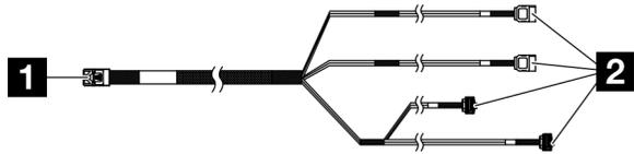
Рис. 111. Mini SAS HD X4 Vertical to VT SATA 7P x2 + RA SATA 7P x2 cable
