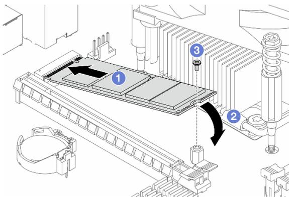
Figure 64. Installing M.2 drive 1
