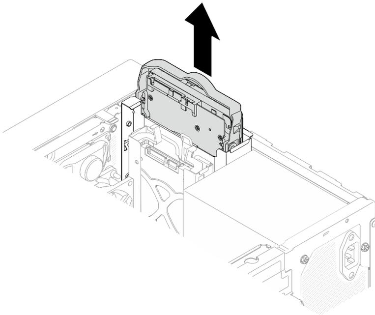
Figure 4. Removing drive assembly from drive bay 0
