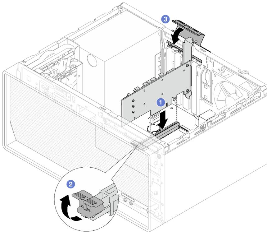
Figure 79. Installing a PCIe adapter
