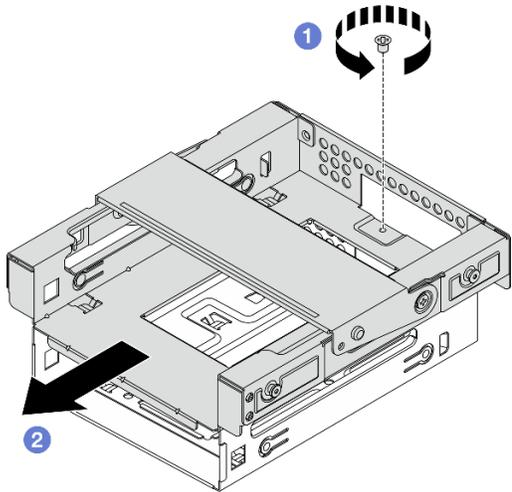
Figure 37. Removing the bay 3 drive cage
