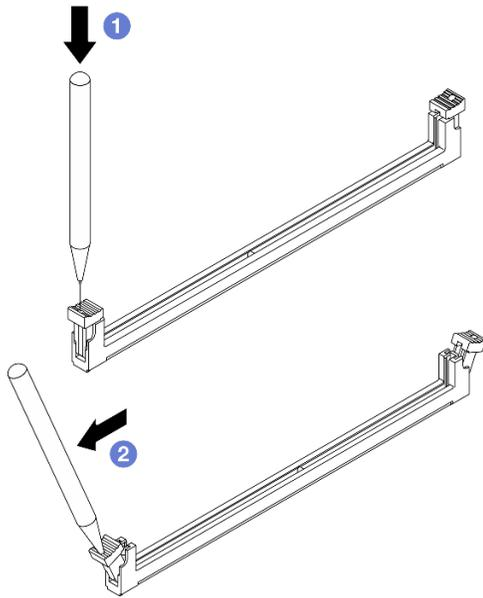
Step 3. Remove the memory module from the slot.
