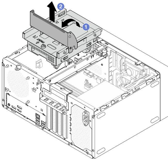
Figure 25. Removing the ODD+bay 2 drive cage assembly
