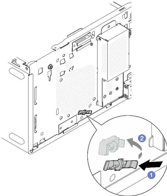
Figure 106. Removing the thermal sensor
