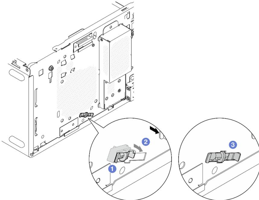
Figure 107. Installing the thermal sensor
