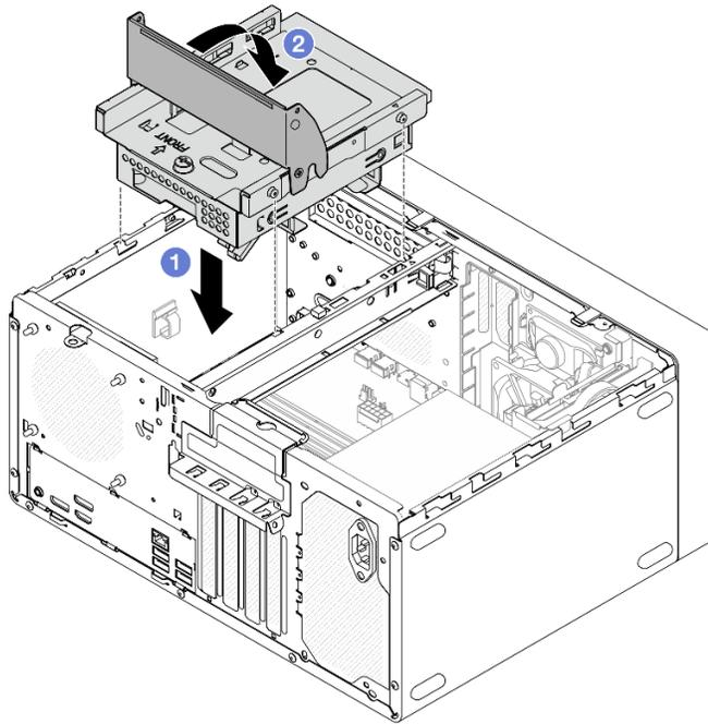
Figure 53. Installing the ODD+bay 2 drive cage assembly
