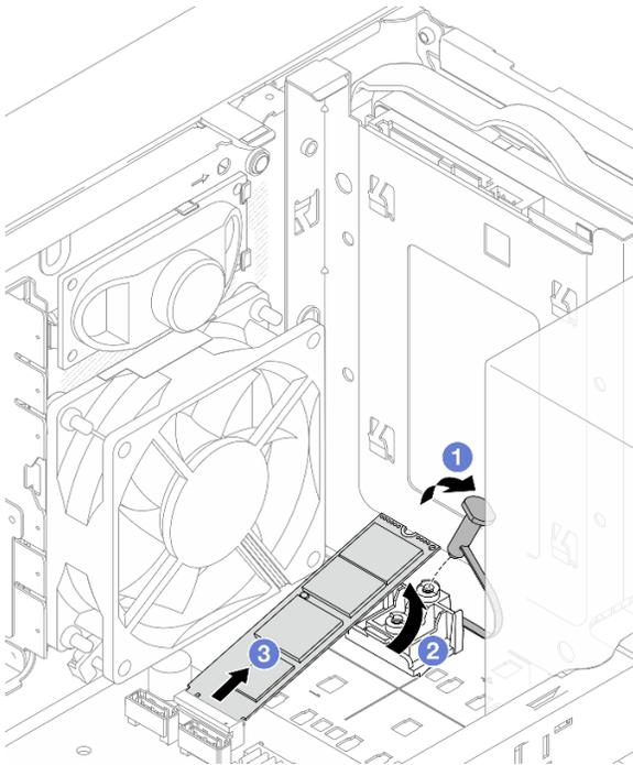
Figure 63. Removing M.2 drive 2
