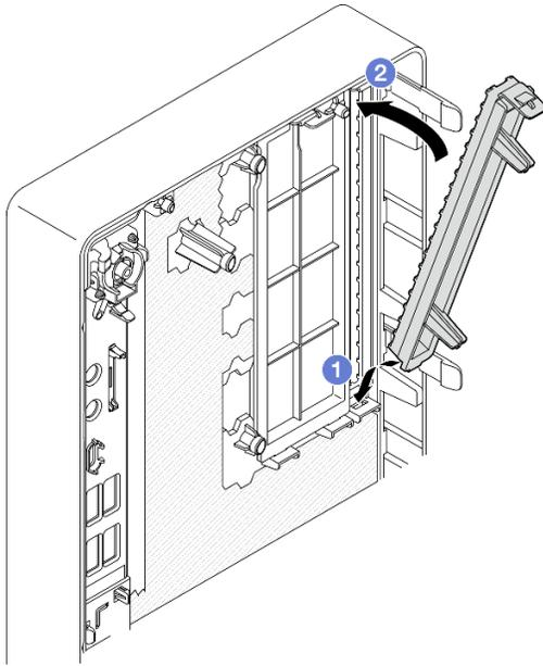
Figure 44. Installing the optical drive bay shield
