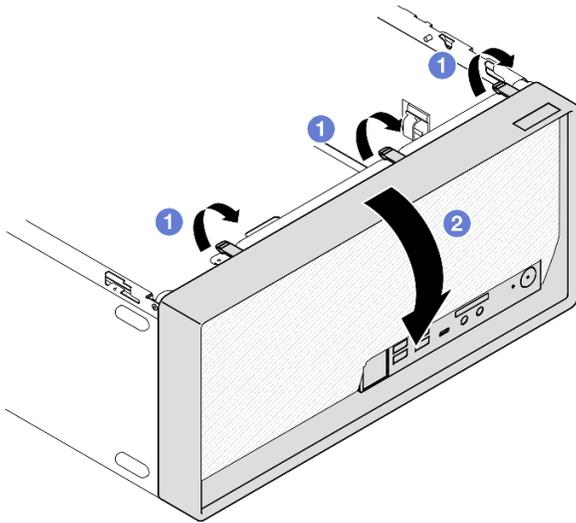
Figure 58. Removing the front bezel
