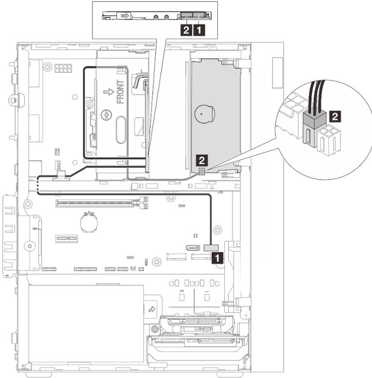
Figure 112. Cable routing for optical disk drive
