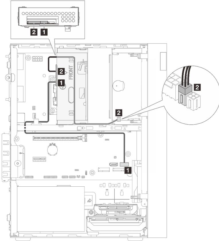
Figure 111. Cable routing for bay 2 drive
