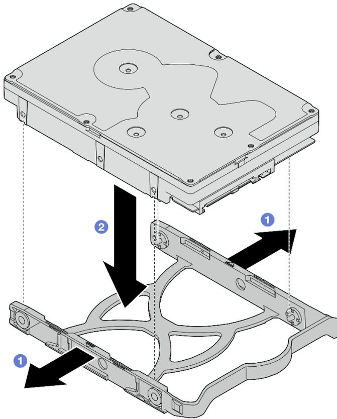
Figure 9. Installing a 3.5-inch drive into the retainer
