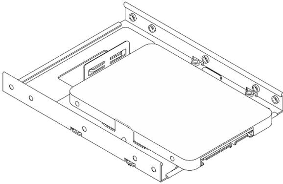
Make sure the screw holes that are nearest to the drive connector are **outside** of the drive retainer.
