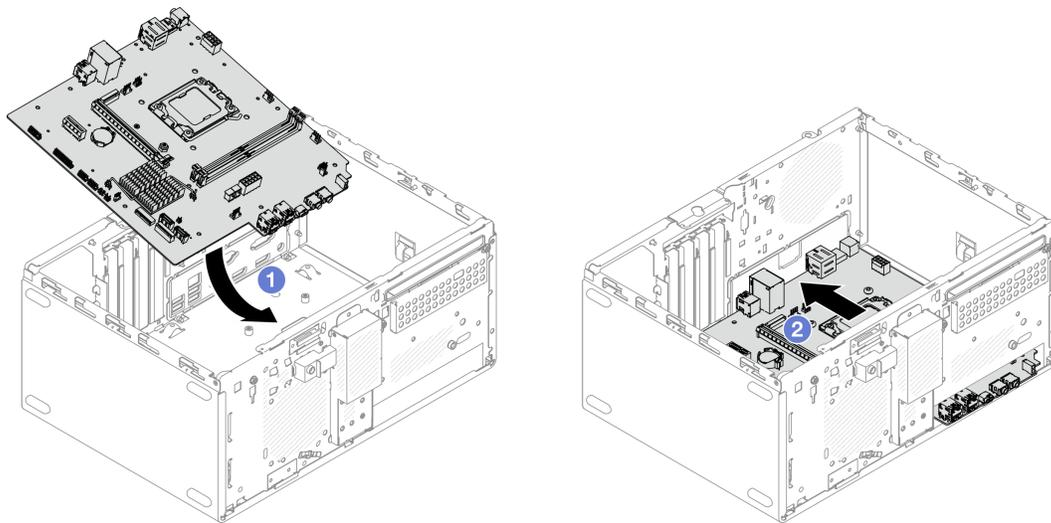
Figure 98. Installing the system board into the chassis
