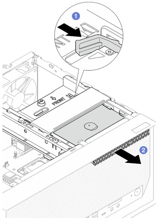
Figure 41. Removing the optical drive
