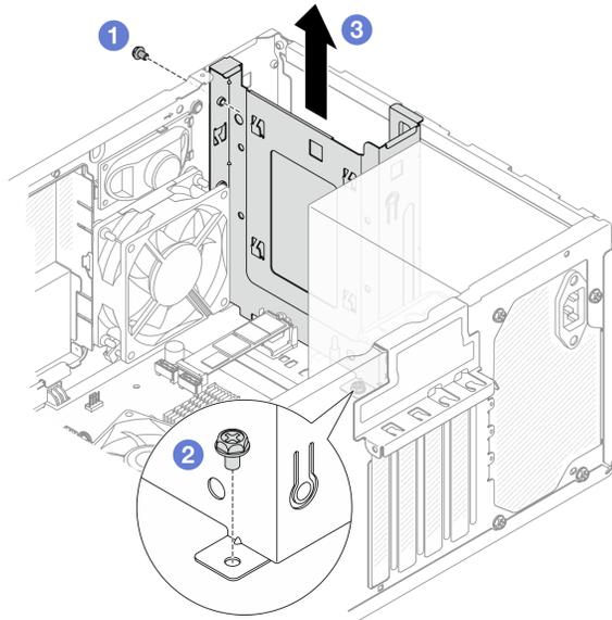
Figure 15. Removing the bay 0 drive cage
