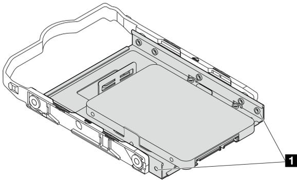
Figure 23. Drive screw hole placement on retainer
