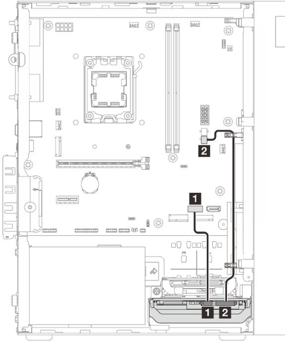
Figure 110. Cable routing for bay 0 drive
