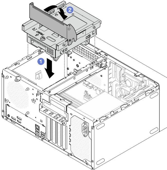
Figure 29. Installing the ODD+bay 2 drive cage assembly
