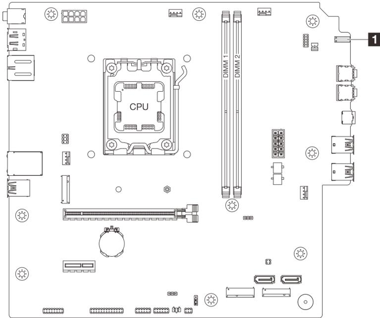
Figure 120. System-board LED
