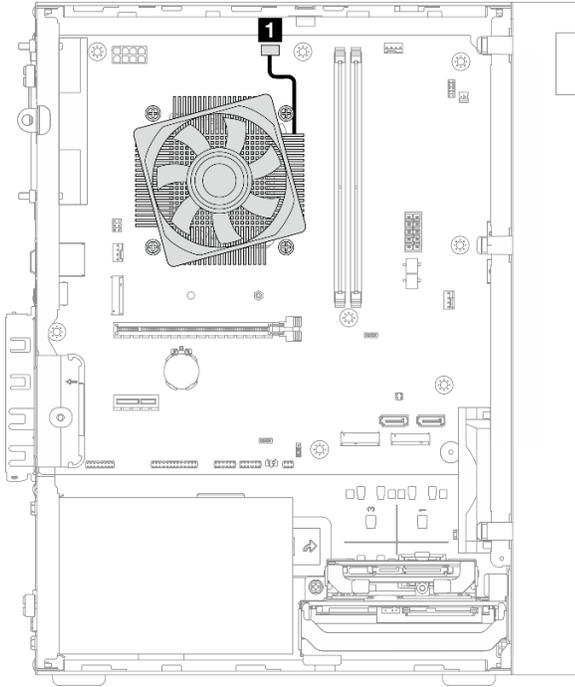
Figure 116. Cable routing for the heat sink and fan module
