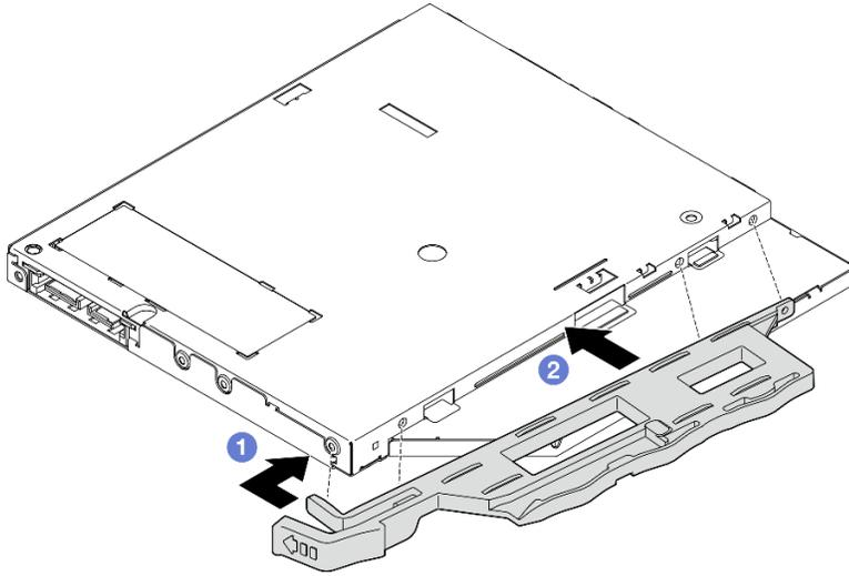
Figure 46. Installing the retainer to the optical drive
