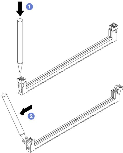
Step 3. Install the memory module into the slot.
