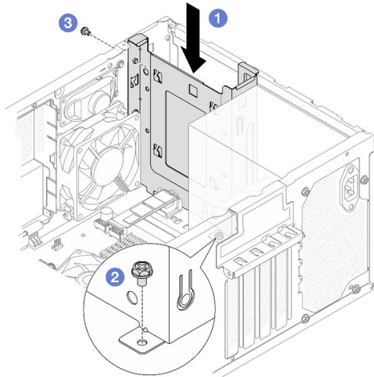
Figure 16. Installing the bay 0 drive cage
