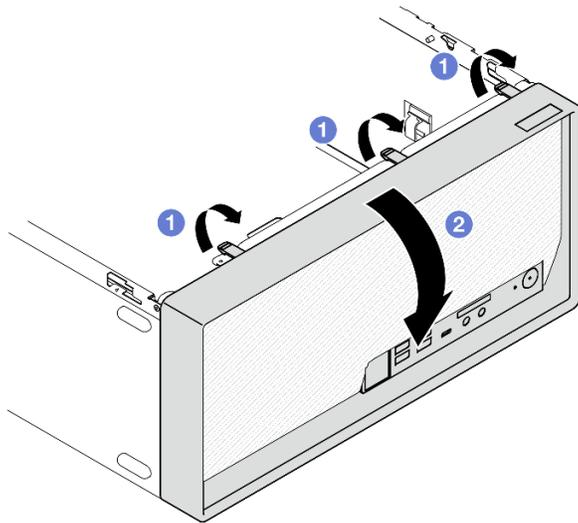
Figure 14. Removing the front bezel
