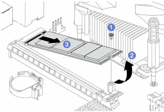
Figure 62. Removing M.2 drive 1
