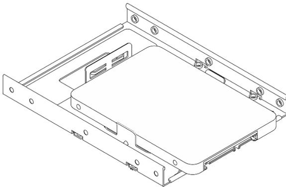
**Remove a 2.5-inch drive from the retainer**
