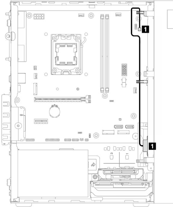
Figure 118. Cable routing for the mono amplifier
