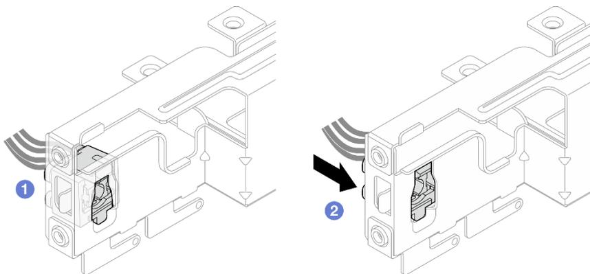
Figure 83. Installing the power button with LED
