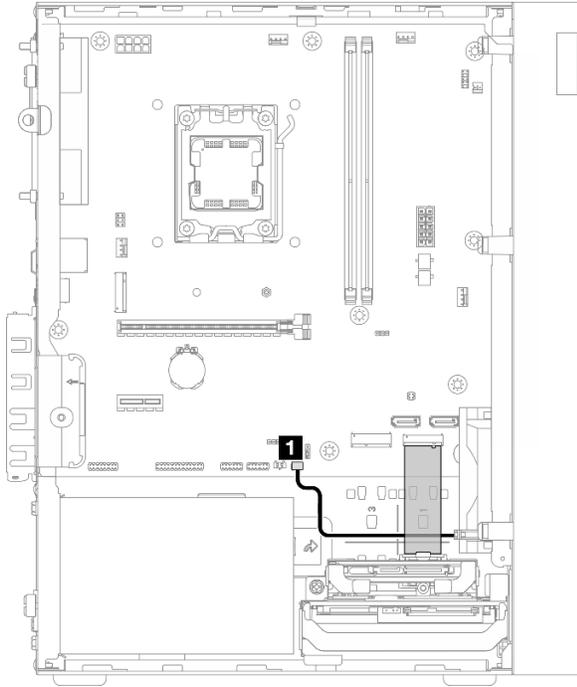
Figure 117. Cable routing for the thermal sensor
