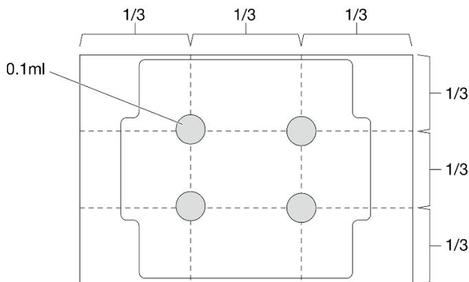
Figure 91. Proper shape of the thermal grease
