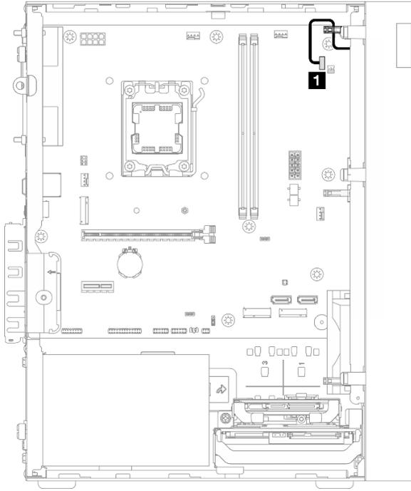
Figure 119. Cable routing for the power button with LED
