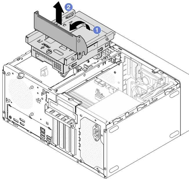
Figure 19. Removing the ODD+bay 2 drive cage assembly
