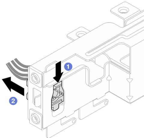
Figure 82. Removing the power button with LED
