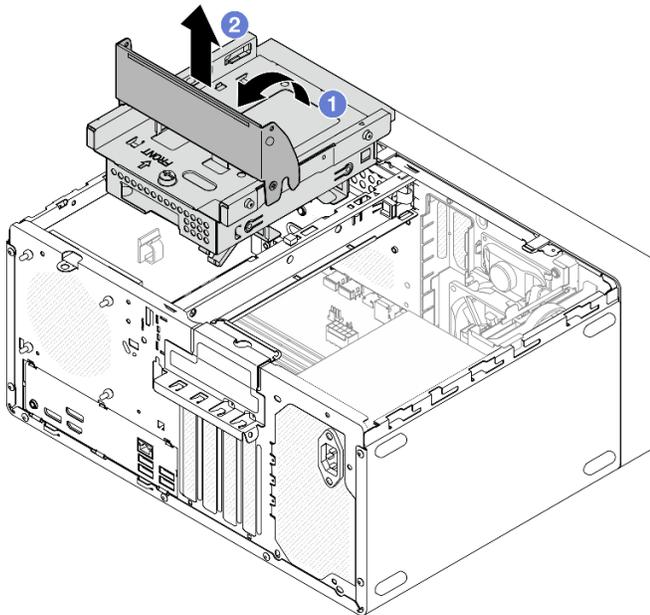
Figure 49. Removing the ODD+bay 2 drive cage assembly
