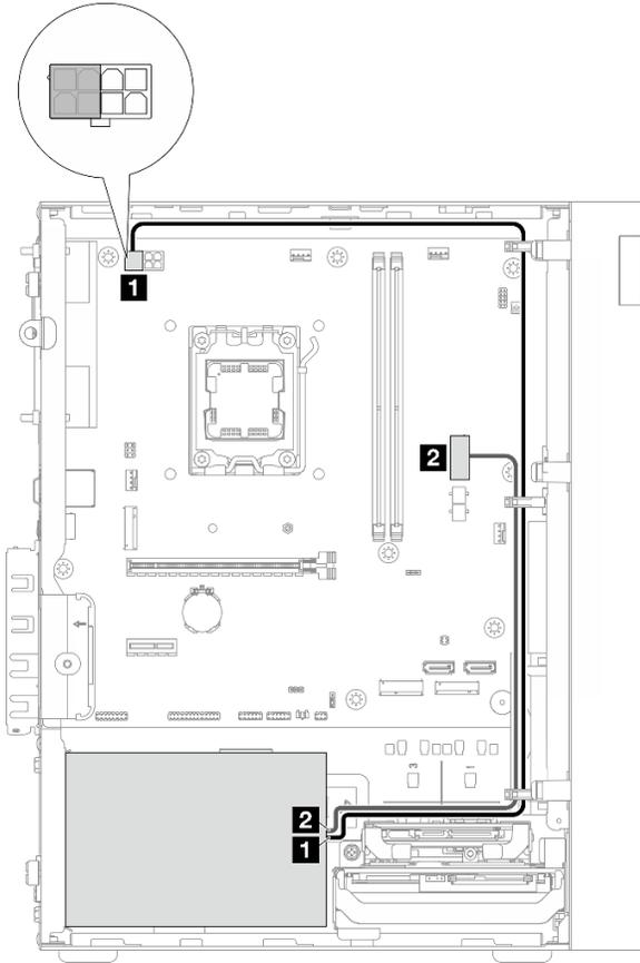
Figure 114. Cable routing for PSU
