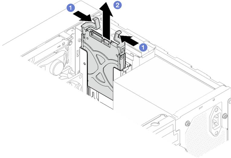
*Figure 5. Removing drive assembly from drive bay 1*
