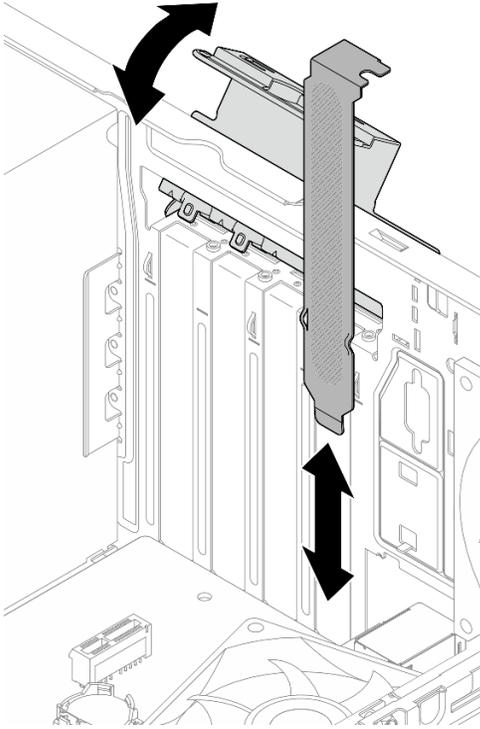
Figure 77. Installing a PCIe adapter bracket
