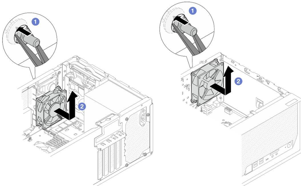
Figure 54. Removing the fan by squeezing rubber mounts
