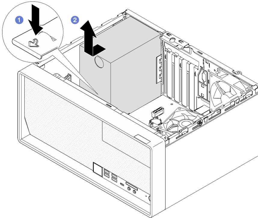
Figure 87. Removing the power supply unit
