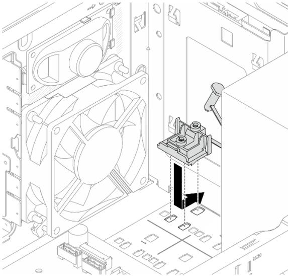
*Figure 67. Installing the M.2 drive retainer*
