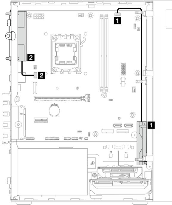
Figure 115. Cable routing for the front fan and rear fan
