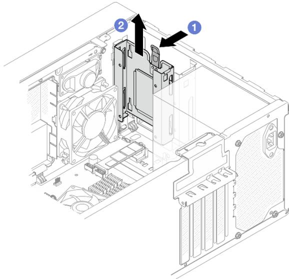
Figure 13. Removing the bay 1 drive cage
