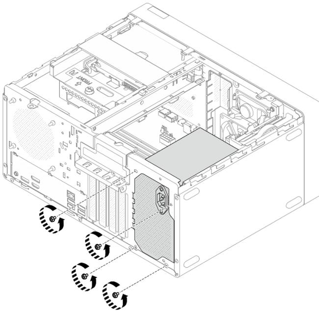
Figure 89. Securing the power supply unit to the chassis
