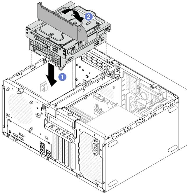
Figure 35. Installing the bay 2+bay 3 drive cage assembly
