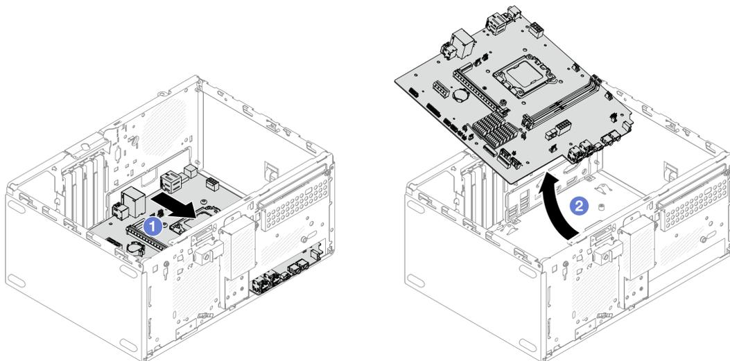
Figure 97. Removing the system board from the chassis
