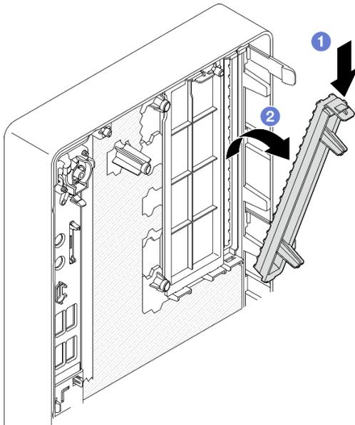
Figure 45. Removing the optical drive bay shield
