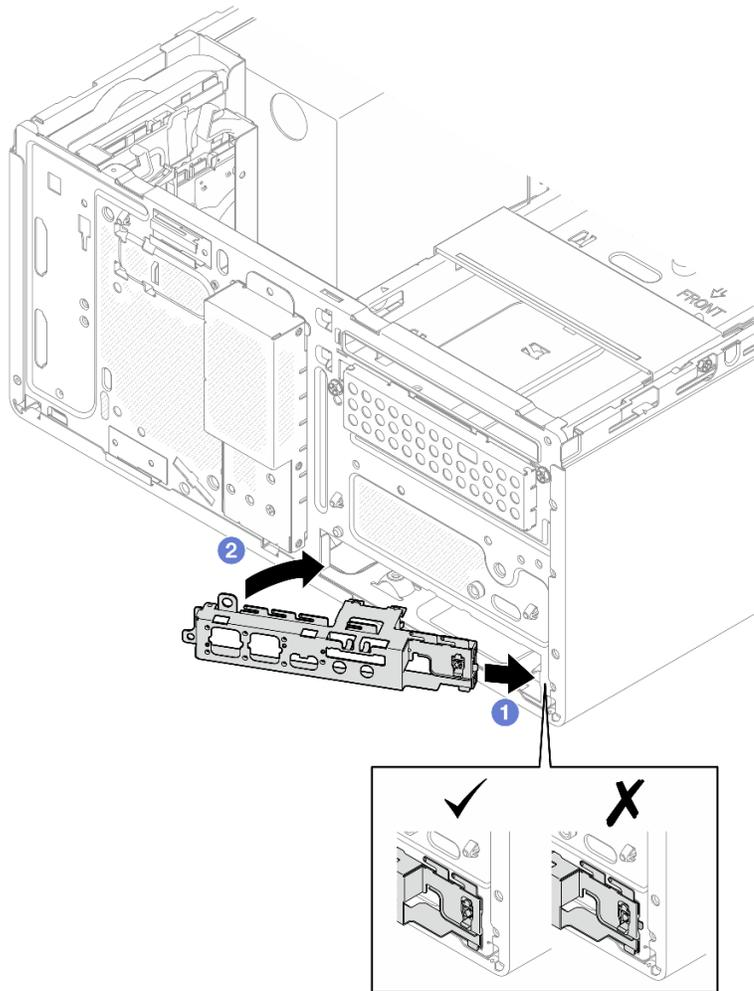
Figure 100. Installing the front I/O bracket to the chassis
