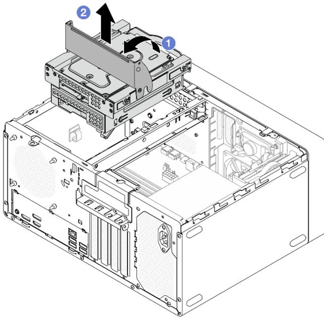
Figure 36. Removing the bay 2+bay 3 drive cage assembly
