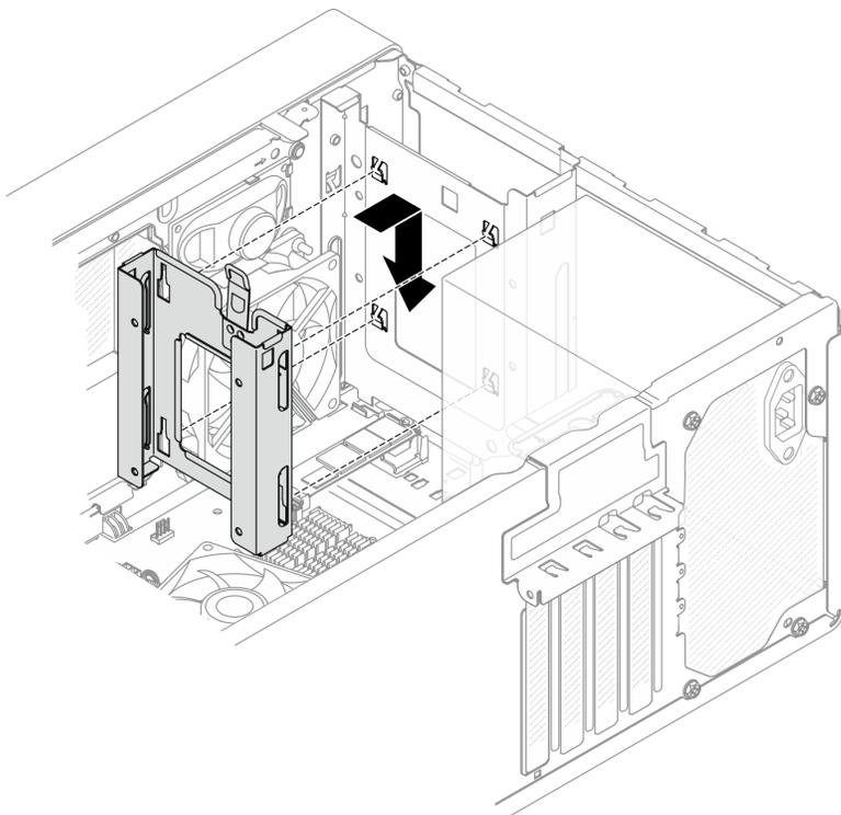
Figure 18. Installing the bay 1 drive cage
