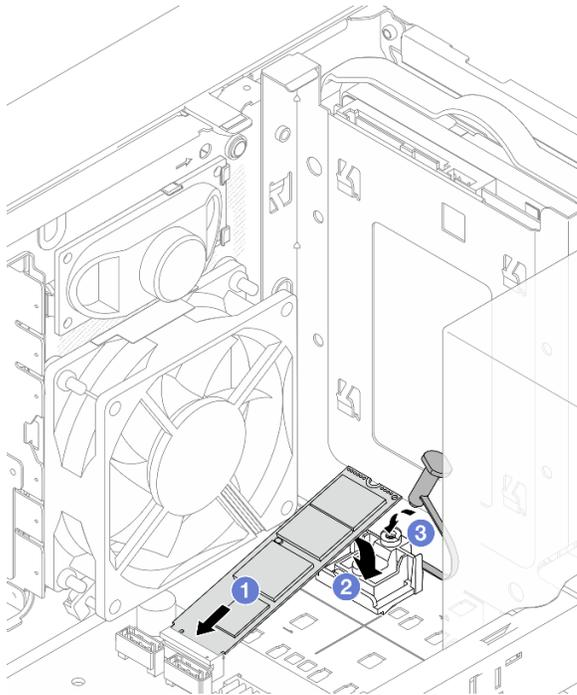
Figure 65. Installing M.2 drive 2
