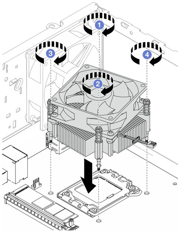
Figure 61. Installing the heat sink and fan module
