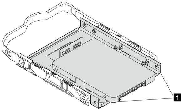
Figure 34. Drive screw hole placement on retainer
