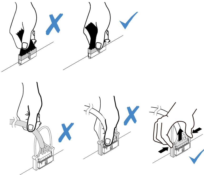
Figure 109. Squeezing the release tabs at both sides to disengage the connector
