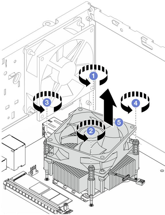
Figure 60. Removing the heat sink and fan module
