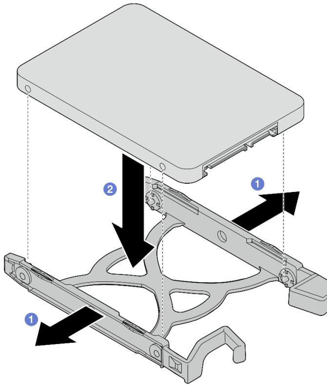
*Figure 10. Installing a 2.5-inch drive into the retainer*
