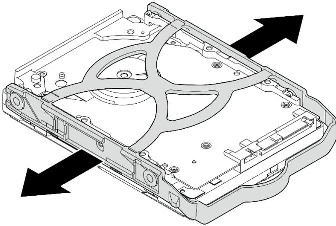
*Figure 6. Removing a 3.5-inch drive from the retainer*
