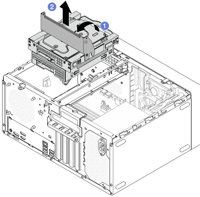
Figure 30. Removing the bay 2+bay 3 drive cage assembly
