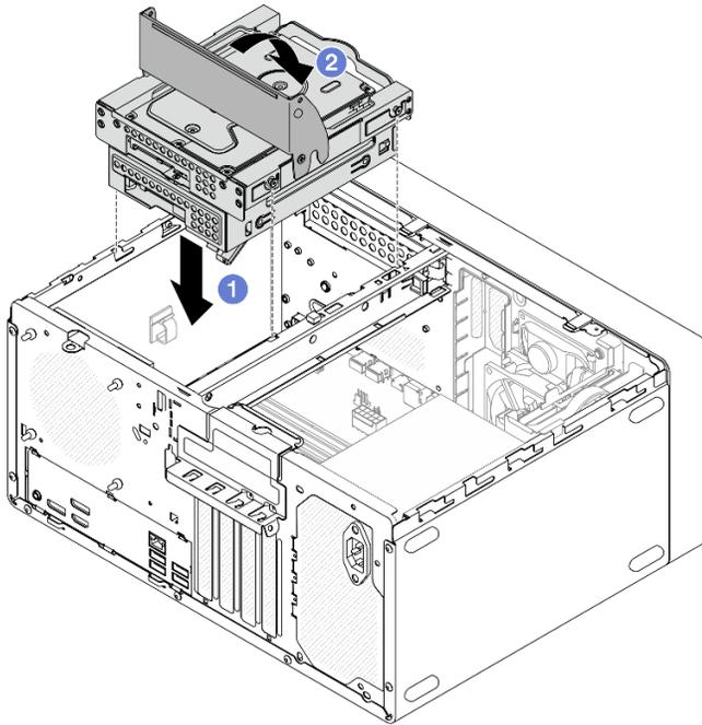
Figure 40. Installing the bay 2+bay 3 drive cage assembly
