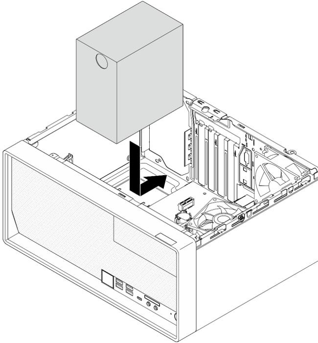
Figure 88. Installing the power supply unit to the chassis
