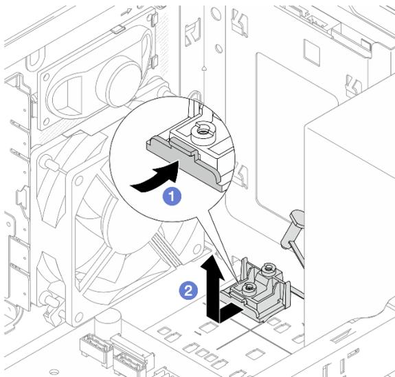
Figure 66. Removing the M.2 drive retainer
