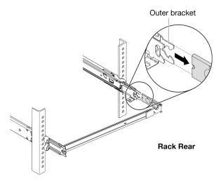
Step 6. Remove the support bar from the rail.
