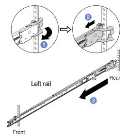
Step 12. Repeat **Step 10 to Step 11** to remove the right rail from the rack.
