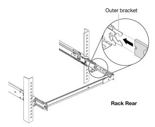
Step 10. Connect the CMA mounting brackets to the rail.
