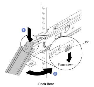
Step 9. Connect the mounting bracket on the support bar to the outer mounting bracket on the rear of the rail.
