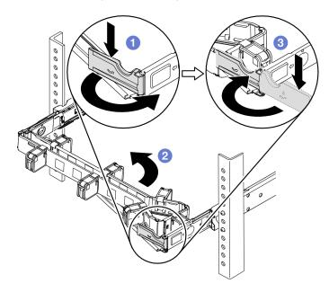
Step 12. Attach the power cords and other cables to the rear of the server. Open the cable brackets on the CMA, route the cables, and then close the cable brackets.
