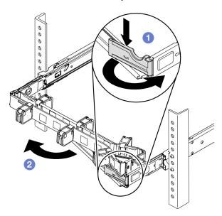
Step 4. Disconnect the CMA mounting brackets from the rail.
