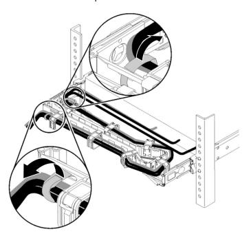
Step 2. Open the cable brackets on the CMA. Then, disconnect the cables from the server and remove them from the CMA.
