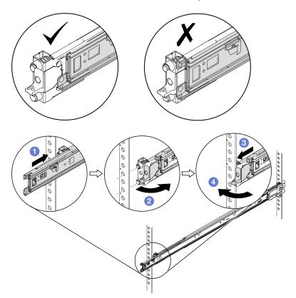
Step 3. Repeat **Step 1 to Step 2** to install the right rail to the opposite side of the rack.
