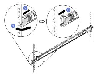
Step 11. Remove the **rear** mounting bracket of the left rail from the front of the rack.
