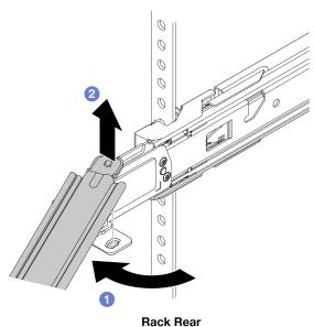
Step 7. Remove the server rack tray from the rails.
