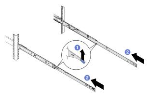
Step 9. If M6 screws are installed into the **rear** of the rails, remove them.
