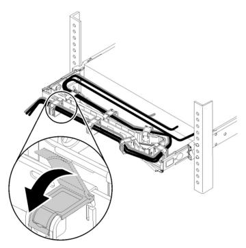
Step 13. Use the cable straps provided to secure the cables. Cables must be bundled with cable straps for proper movement.
