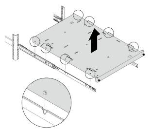
Step 8. Slide the rails into the rack.
