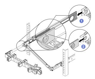
Step 5. Disconnect the mounting bracket on the support bar from the outer mounting bracket on the rear of the rail.
