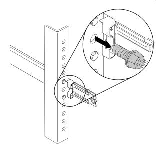
Step 10. Remove the front mounting bracket from the left rail.
