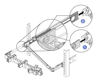
Step 11. Place the CMA onto the support bar and close the stop bracket.
