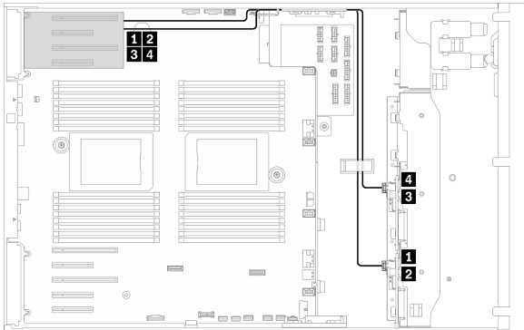
Figure 158. NVMe cable routing to top PCIe zone
