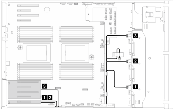
Figure 104. SAS/SATA cable routing to bottom PCIe zone
