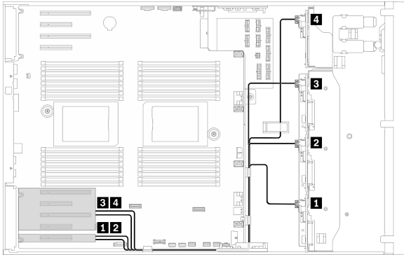
Figure 148. SAS/SATA cable routing to bottom PCIe zone
