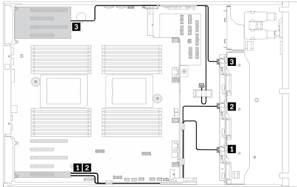
Figure 125. SAS/SATA cable routing to top PCIe zone
