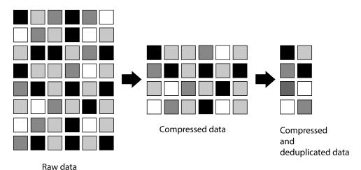
When you run deduplication on a FlexVol volume that contains uncompressed data, it scans all the uncompressed blocks in the FlexVol volume and creates a digital fingerprint for each of the blocks.
