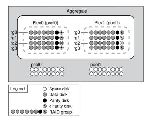
The following diagram shows an aggregate composed of array LUNs with the SyncMirror functionality enabled and implemented. A second plex has been created for the aggregate, plex1. Plex1 is a copy of plex0, and the RAID groups are also identical.
