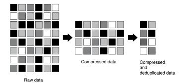
When you run deduplication on a FlexVol volume that contains uncompressed data, it scans all the uncompressed blocks in the FlexVol volume and creates a digital fingerprint for each of the blocks.
