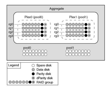
The following diagram shows an aggregate composed of array LUNs with the SyncMirror functionality enabled and implemented. A second plex has been created for the aggregate, plex1. Plex1 is a copy of plex0, and the RAID groups are also identical.
