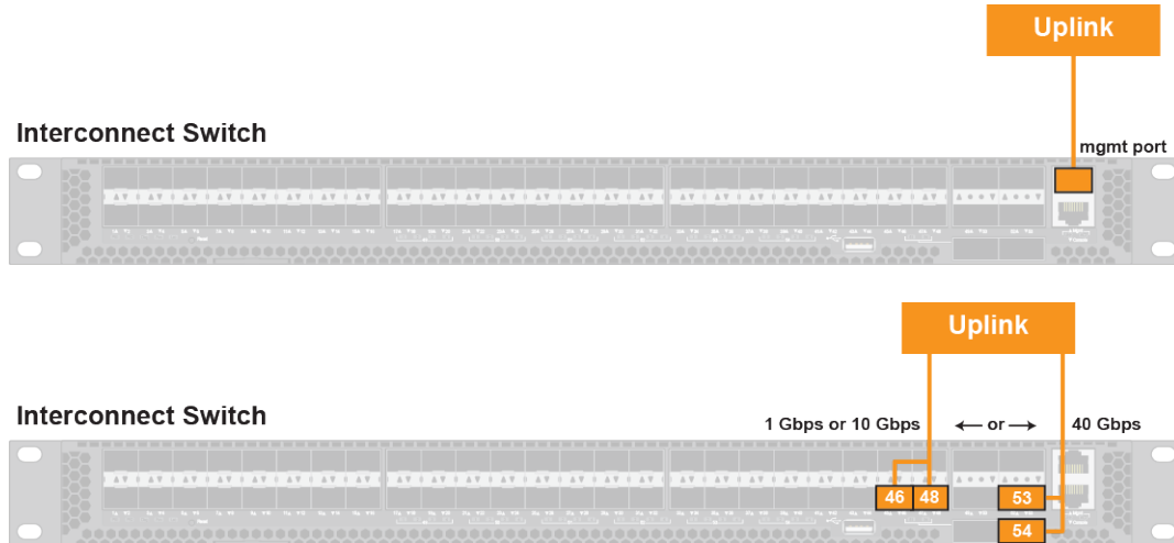
Figure 33. Customer data center connection: dual direct link
