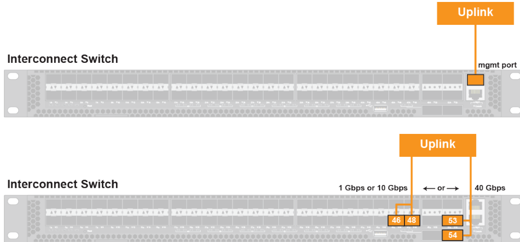
Figure 35. Customer data center connection: LAG direct link
