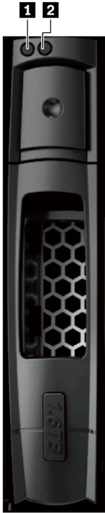
Figure 55. LEDs on the 2.5-inch drives
