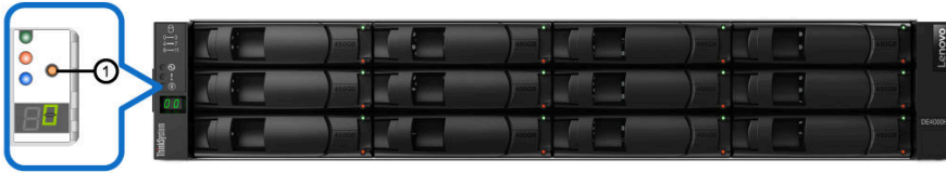
Figure 52. ODP push button on controller shelf and drive shelf with 12 drives
