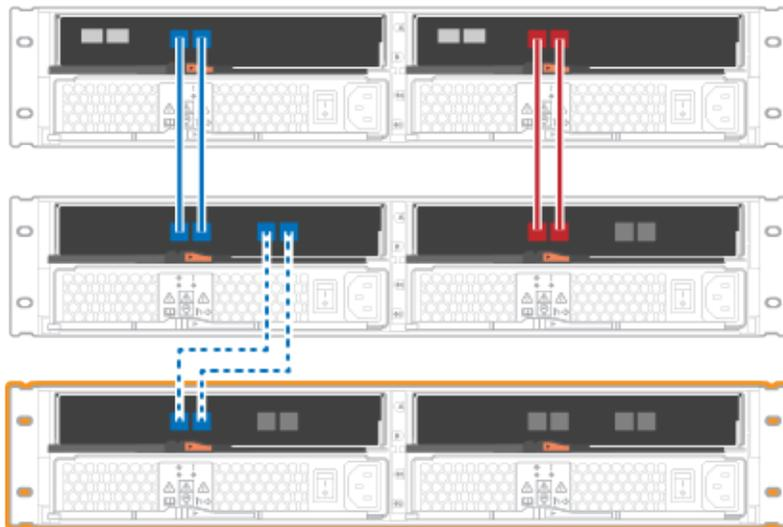
Figure 12. Single-stack diagram (2U models)
