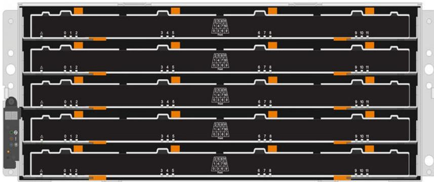
For both a DE4000H/DE6000H controller shelf drawer and a DE600S drive shelf drawer, drives are numbered from 0 to 11 in each drive drawer within the shelf.
