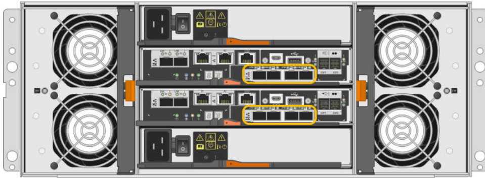
Figure 29. With two 4-port SFP+ (optical) HICs (4U)
