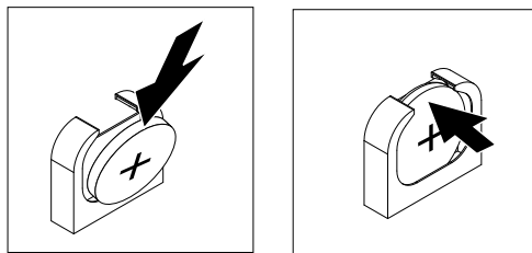
Figure 232. System battery installation
