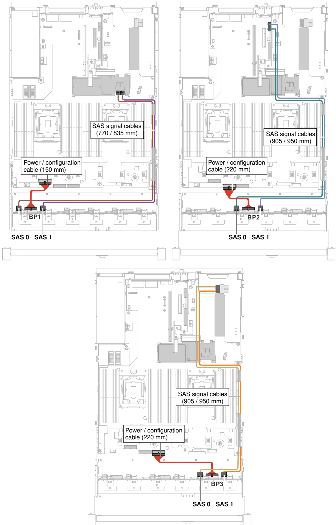
138 Figure 61. 24x2.5-inch hot-swap hard disk drive cabling Lenovo System x3650 M5 Installation and Service Guide
