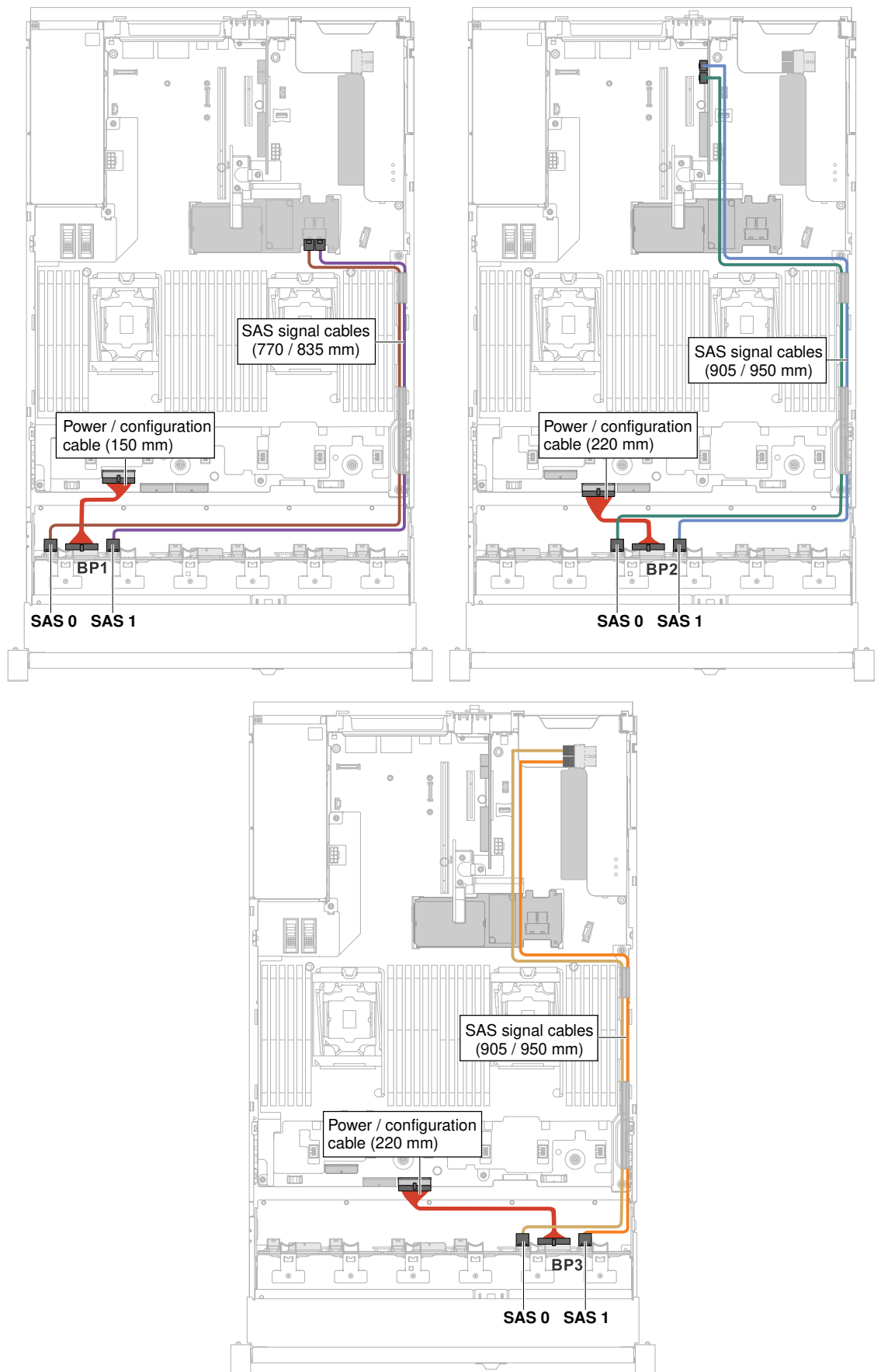
Figure 274. Cable routing
