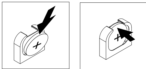
Figure 208. System battery installation
