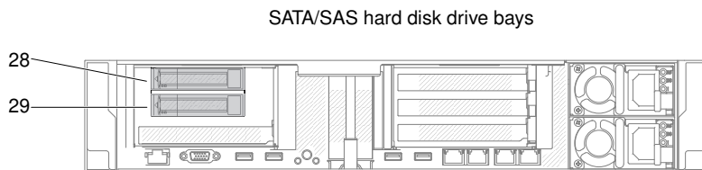
Figure 139. One 2.5-inch rear two hard-disk-drive kit numbering
