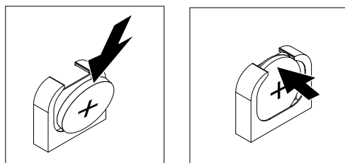
Figure 215. Coin-cell battery installation
