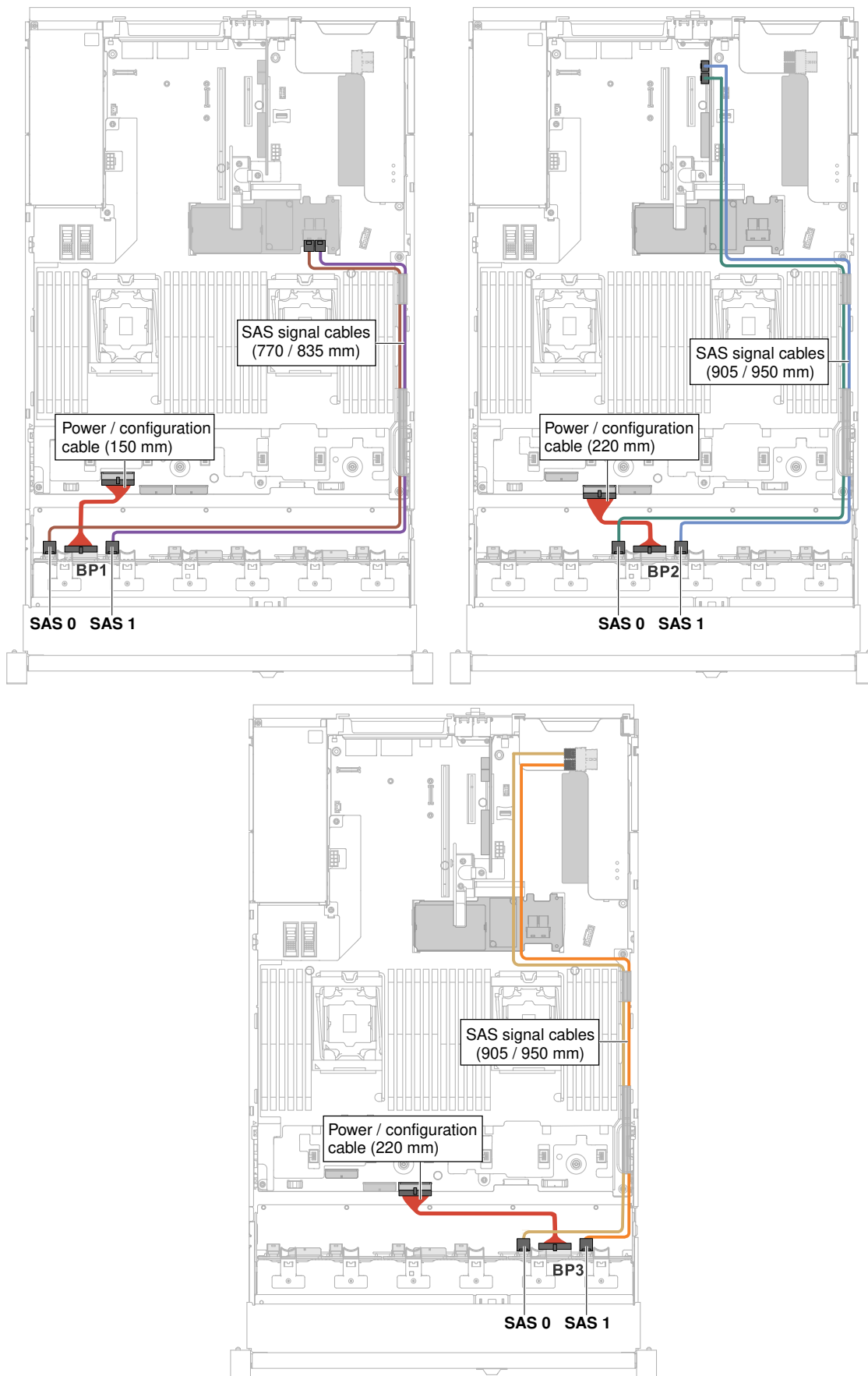
Figure 68. 24x2.5-inch hot-swap hard disk drive cabling
