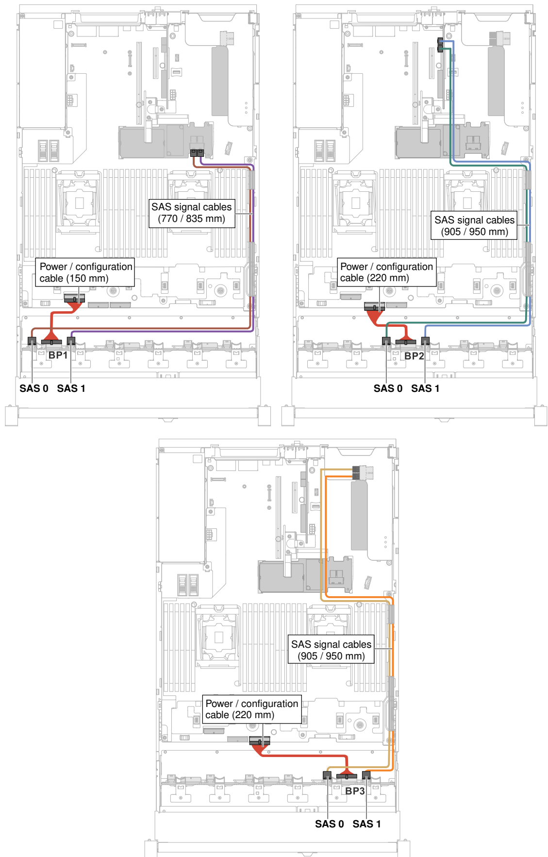
Figure 281. Cable routing
